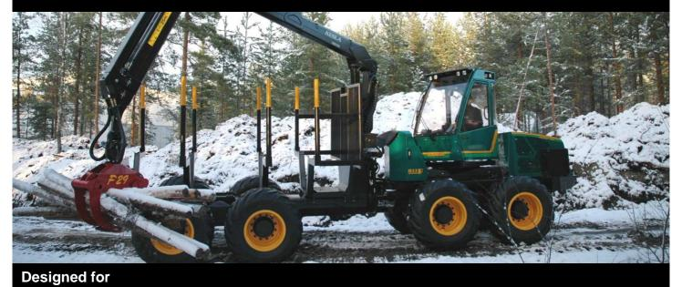
**KESLA 29** grapple is designed for medium size forwarders. This grapple type is also used with small timber cranes.
