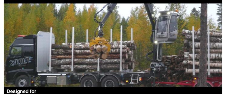
**KESLA 46** grapple is our recommendation, when loading pulp wood and large stocks. 46 grapple is suitable for both mobile and stationary cranes.
