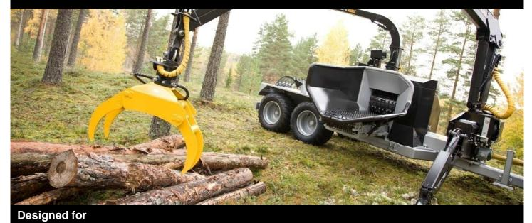
**KESLA15E** energy wood grapple is designed for handling mixed silage and energy wood. Fast opening and closing of jaws combined with light weight have made this grapple popular. It is an excellent combination with chippers and energy wood trailors.
