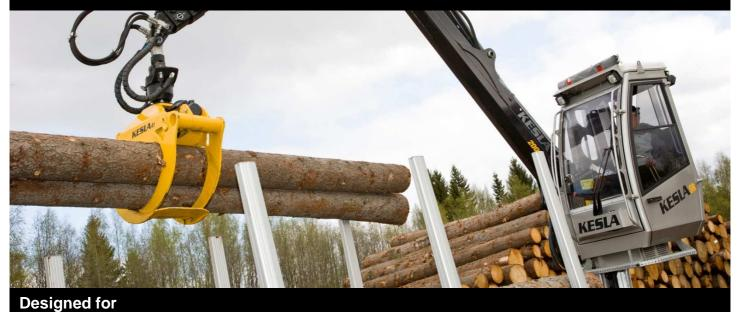
**KESLA 41** timber grapple is designed to be all-purpose timber grapple. It is suitable for both pulp and saw wood stocks. Kesla 41 is our recommendation, when you have 10-14 mtn loader and all timber sortiments to load.
